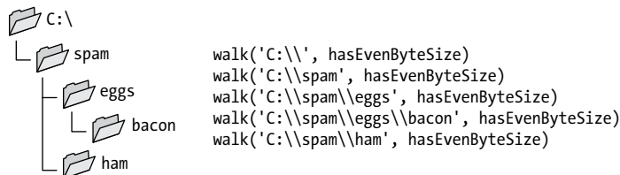
Figure 10-1: An example filesystem and the recursive walk() function calls over it
