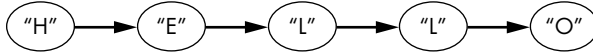
Figure 4-3: A linked list data structure storing HELLO . Linked lists can be considered a kind of tree data structure.
